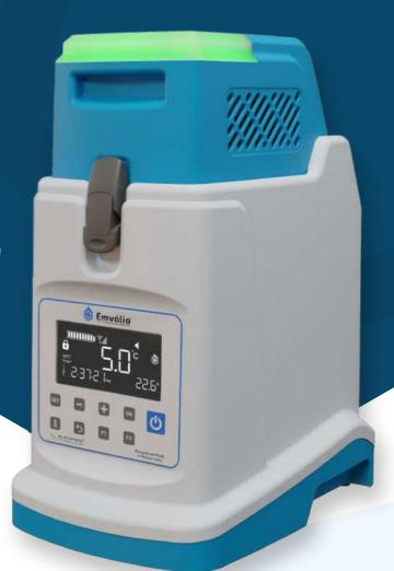
Emvólio is a Portable active-cooling (battery-powered) device that will provide a platform for delivery of vaccines and all other biologicals like blood, serums, viral culture which require to be kept strictly between 2°C and 8°C for 12+ hours in the field. The product has been designed in accordance with WHO PQS E003 specifications and conforms to IEC 60601 standards.
